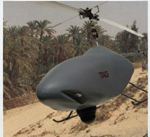
▲ The TAG-M80 improvements include integrating all mechanics and electronics into the interior of the fuselage and tail boom.
